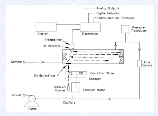
This measuring principle corresponds to the standard reference method as described in EN 14626.
