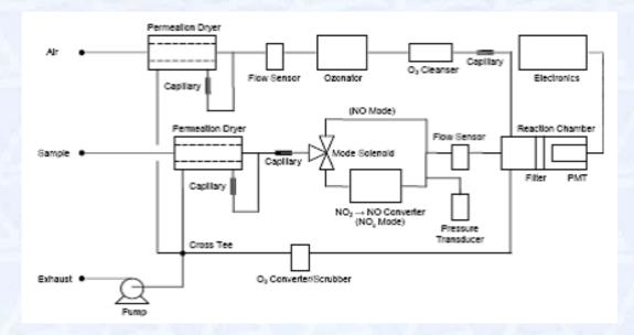
This measuring principle corresponds to the standard reference method as described in EN 14211.
