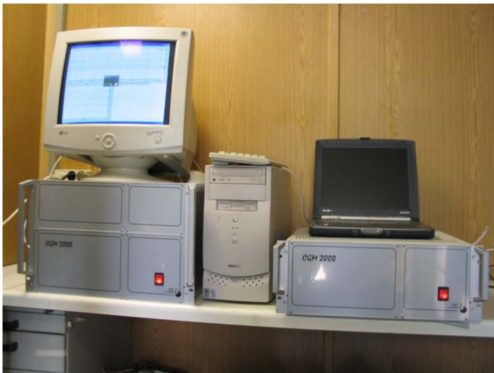
Figure 4: Set up of the ozone generator and the computer for controlling
