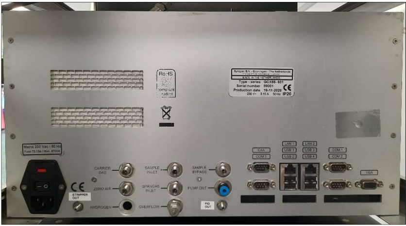
Fig. 2.2: Rear view of the gas chromatograph
