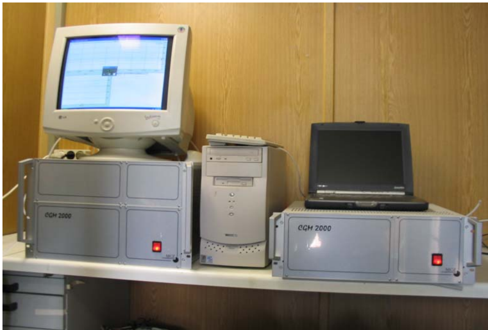
Figure 4: Set up of the sulphur dioxide generator and the computer for controlling
