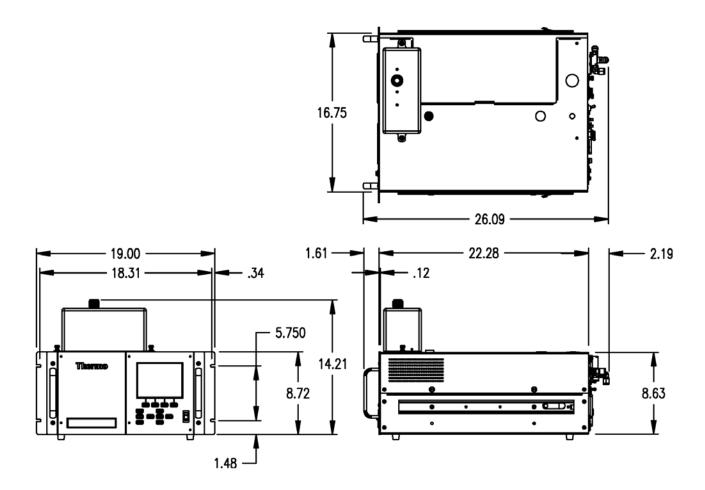
Figure 9–2. EIA Rack Mounting
