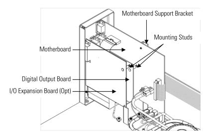
Figure 7–13. Replacing the I/O Expansion Board (Optional)
