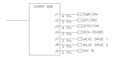
Figure 6–3. Board-Level Connection Diagram - SHARP
