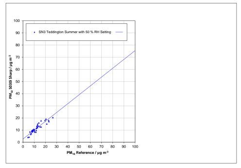
**Figure 26:** Comparison of reference and candidate SN 3, measured component PM<sub>10</sub>, Teddington (summer), relative humidity threshold adjusted to 50 %
