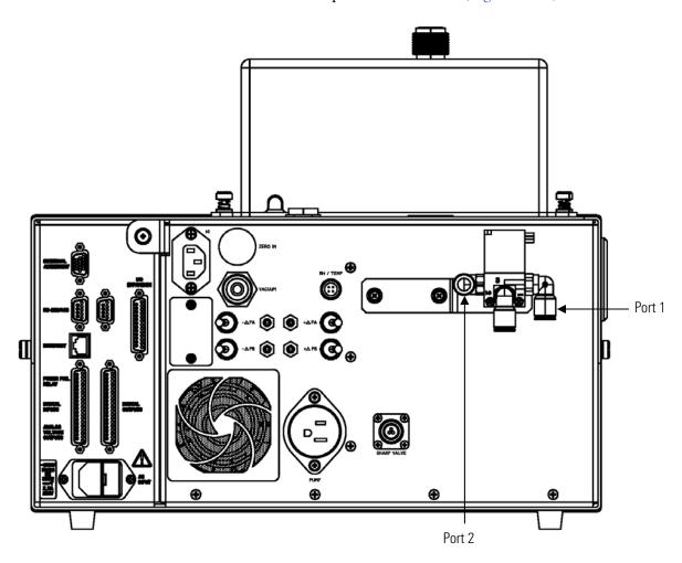
**Figure 10–7.** Rear Valve Assembly Installation
