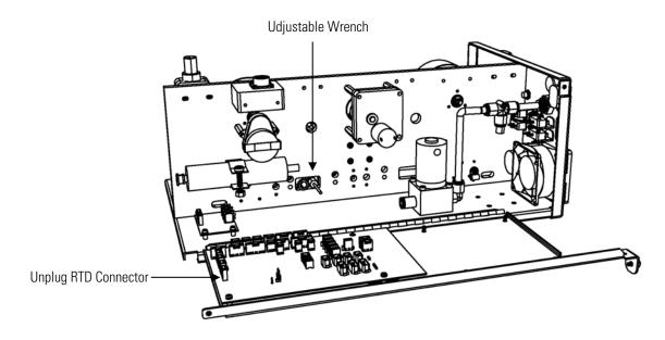
Figure 7–19. Replacing the RTD
