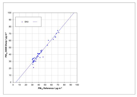
Figure 74: Reference vs. candidate, SN 3, measured component PM<sub>10</sub>, values ≥ 30 μg/m³
