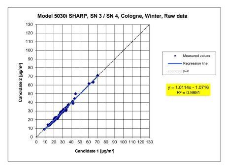
**Figure 57:** Results of the parallel measurements with the candidates SN 3 / SN 4, measured component PM<sub>10</sub>, test site Cologne (winter)
