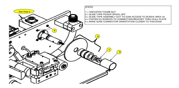
Figure 10–2. Tape Pick-up Spool Removal
