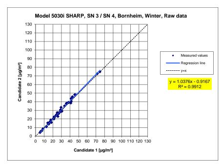
**Figure 59:** Results of the parallel measurements with the candidates SN 3 / SN 4, measured component PM<sub>10</sub>, test site Bornheim (winter)
