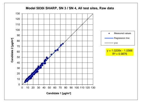
**Figure 56:** Results of the parallel measurements with the candidates SN 3 / SN 4, measured component PM<sub>10</sub>, all test sites
