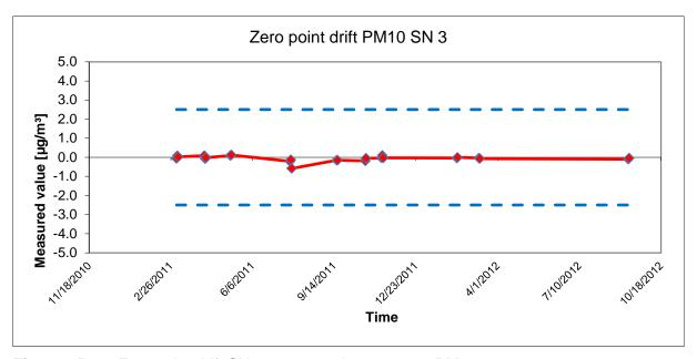
Figure 35: Zero point drift SN 3, measured component PM<sub>10</sub>
