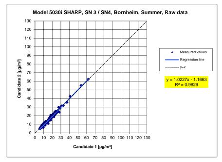
**Figure 58:** Results of the parallel measurements with the candidates SN 3 / SN 4, measured component PM<sub>10</sub>, test site Bornheim (summer)
