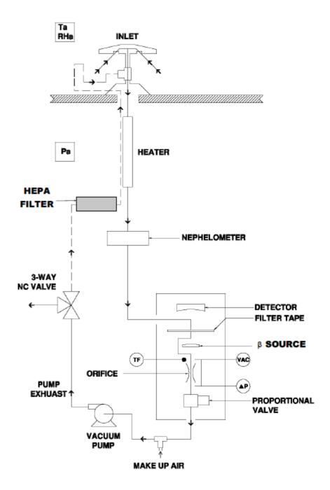
Figure 5: Diagram – Set-up of Model 5030i SHARP
