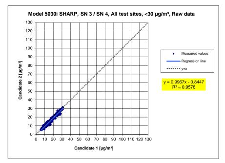
Figure 62: Results of the parallel measurements with the candidates SN 3 / SN 4, measured component  $PM_{10}$ , all test sites, values < 30  $\mu g/m^3$
