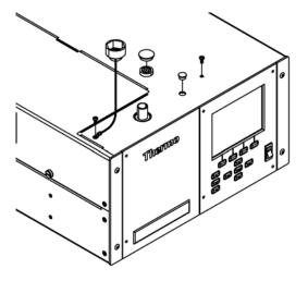
Figure 10–6. Radius Tube Adapter Alignment Check
