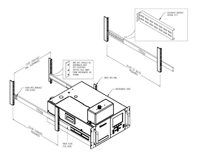
Figure 9-4. Rack Mount Option Assembly
