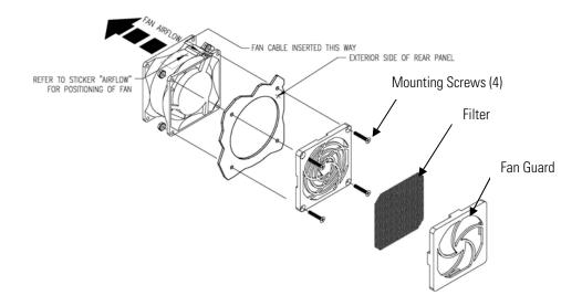
**Figure 5–4.** Inspecting and Cleaning the Fan
