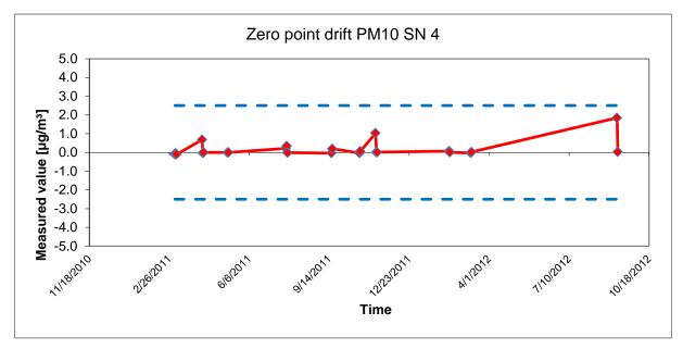
Figure 36: Zero point drift SN 4, measured component PM<sub>10</sub>
