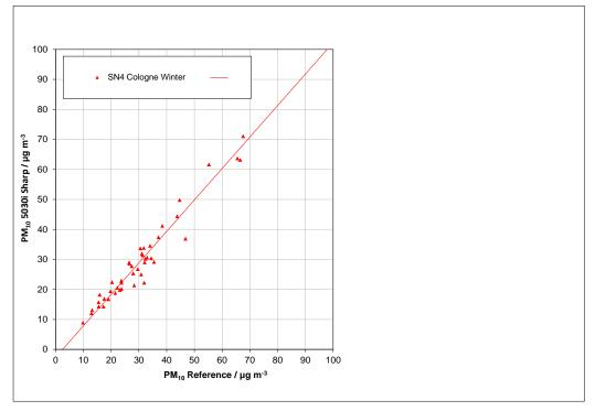
Figure 67: Reference vs. candidate, SN 4, measured component PM<sub>10</sub>, Cologne (winter)
