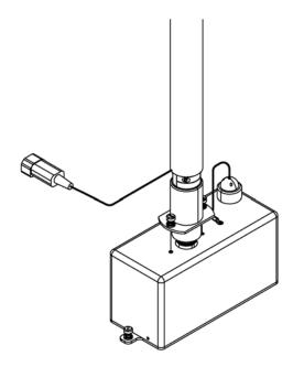
Figure 10-12. Connecting Heater to Optics Assembly Cover
