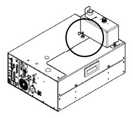
Figure 10–10. Connecting the Optics to the Optics Connector
