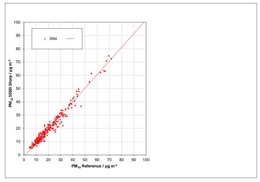
Figure 65: Reference vs. candidate, SN 4, measured component PM<sub>10</sub>, all test sites
