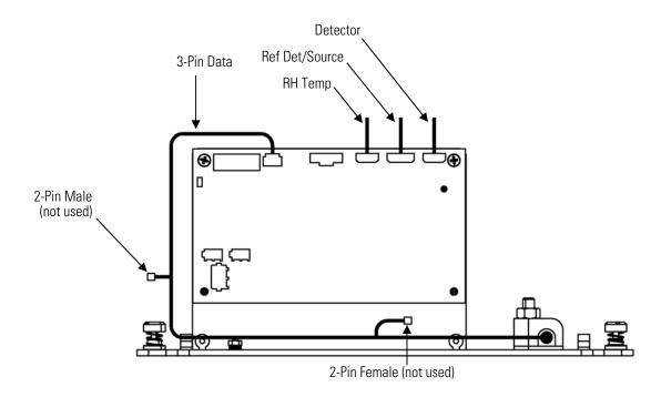
Figure 7–27. SHARP Interface Board Connections
