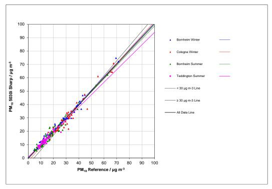
Figure 63: Reference vs. candidate, SN 3 & SN 4, measured component PM<sub>10</sub>, all test sites
