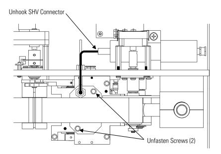
Figure 7–18. Replacing the Detector Assembly
