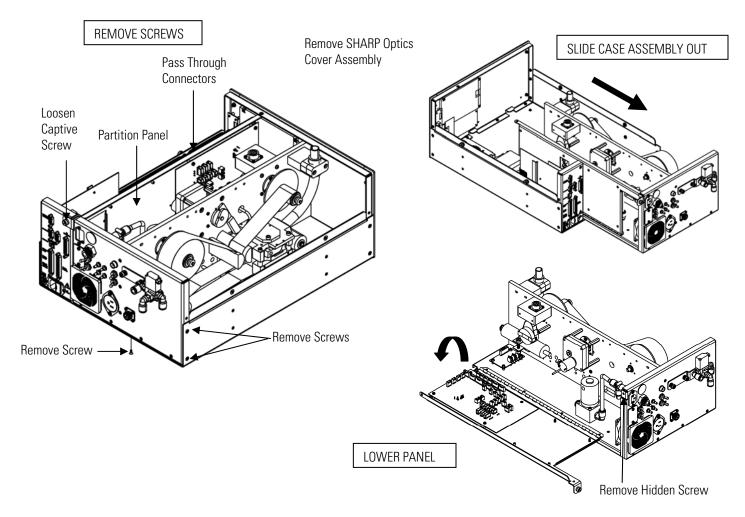
**Figure 7–5.** Removing the Measurement Case Assembly and Lowering the Partition Panel
