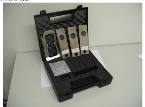
Figure 17: Set with foil holder and test foils
