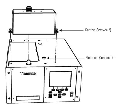
**Figure 7–4.** Removing the SHARP Optics Assembly
