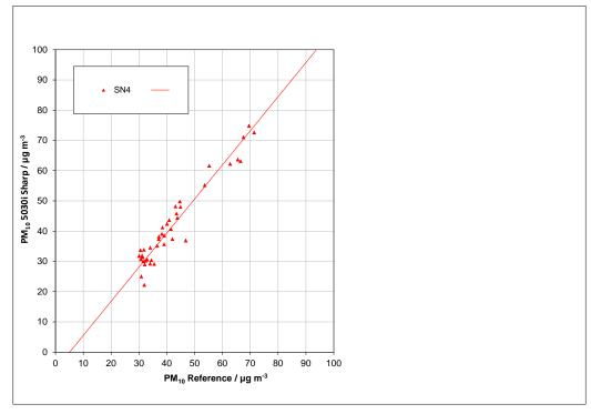
Figure 75: Reference vs. candidate, SN 4, measured component  $PM_{10}$ , values  $\geq 30 \mu g/m^3$
