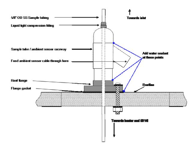
Figure 9–5. Roof Flange Assembly
