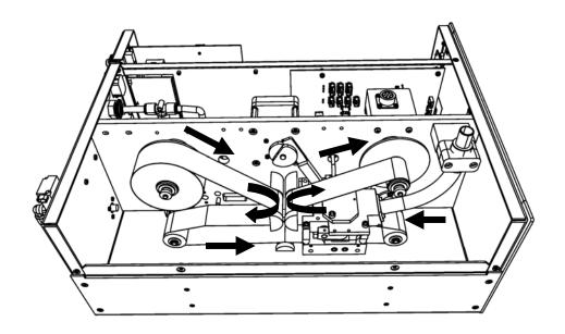
Figure 5–5. Replacing the Filter Tape
