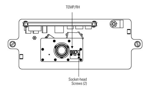
Figure 7–26. Disconnecting the RH/Temp Connector
