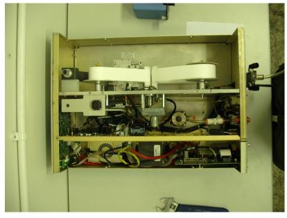
Figure 4: Picture of hardware components Model 5030i SHARP – Beta module
