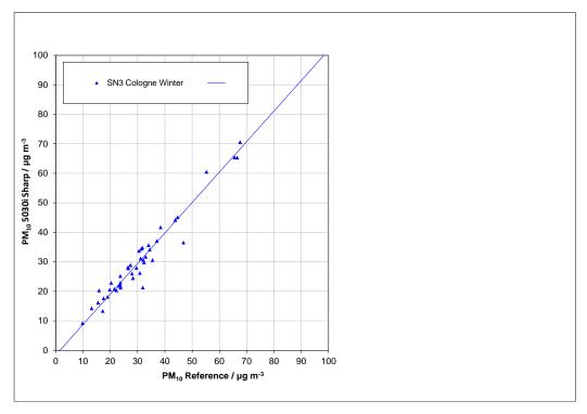
Figure 66: Reference vs. candidate, SN 3, measured component PM<sub>10</sub>, Cologne (winter)
