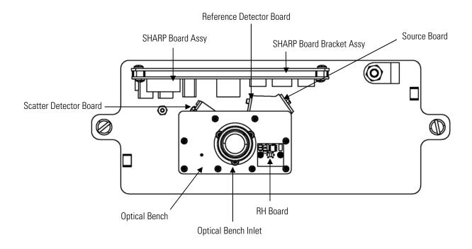
Figure 7–3. SHARP Optics Component Layout
