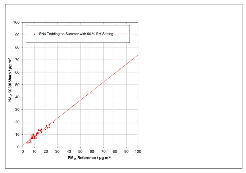
**Figure 27:** Comparison of reference and candidate SN 4, measured component PM<sub>10</sub>, Teddington (summer), relative humidity threshold adjusted to 50 %
