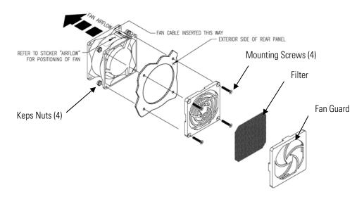
Figure 7–6. Replacing the Fan
