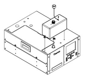
Figure 10–9. Optics Installation
