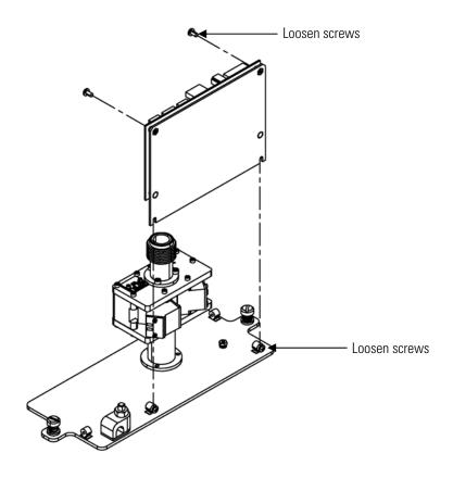
Figure 7–28. Replacing the SHARP Optics Board
