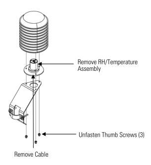
Figure 7–22. Replacing the Ambient RH/Temperature Assembly
