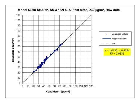
Figure 61: Results of the parallel measurements with the candidates SN 3 / SN 4, measured component  $PM_{10}$ , all test sites, values  $\geq$  30  $\mu g/m^3$
