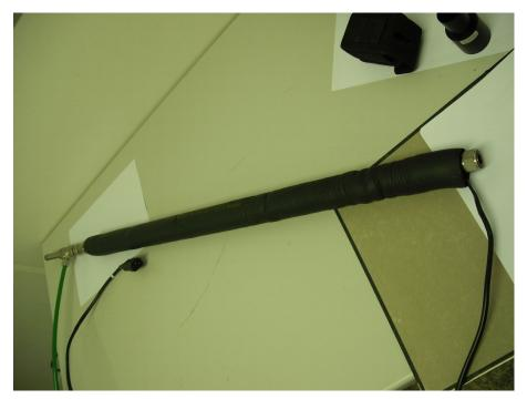
Figure 8: Heated sampling tube (DHS)
