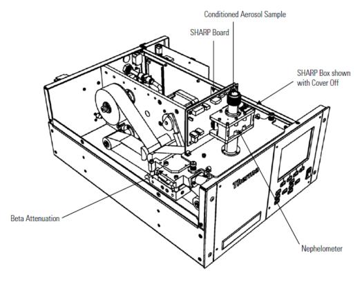
Figure 1: Sample path within the Model 5030i SHARP measuring system
