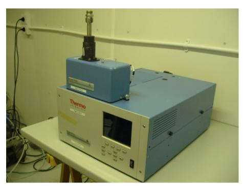
Figure 9: Model 5030i SHARP measuring system
