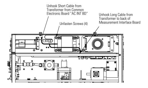
Figure 7–20. Replacing the Transformer
