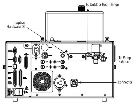
Figure 7–25. Replacing the External Solenoid Valve
