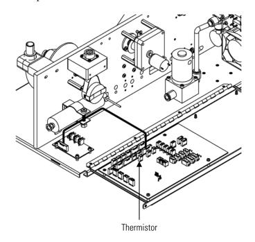
Figure 7–12. Replacing the Thermistor
