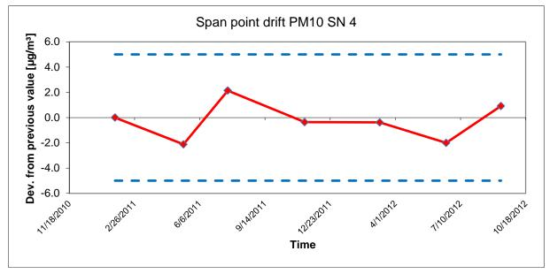
Figure 38: Drift of the measured value SN 4, measured component PM<sub>10</sub>
