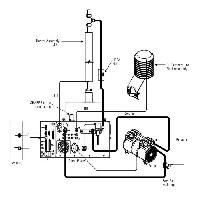
Figure 2–7. Rear Panel Plumbing Schematic
