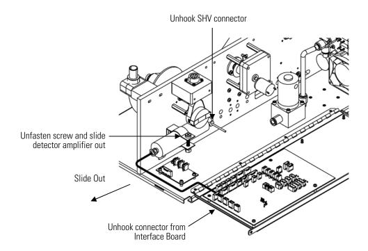
**Figure 7–7.** Replacing the Detector Amplifier Assembly
