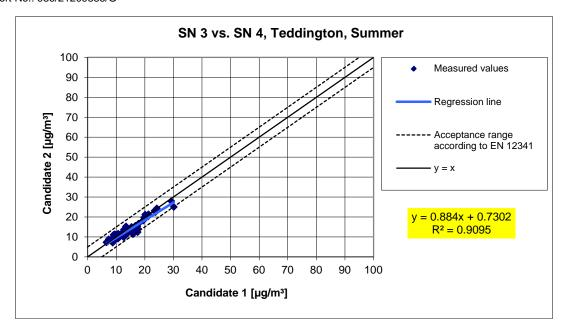
**Figure 52:** Result of parallel measurements with candidates SN 3 / SN 4, Teddington (summer)
