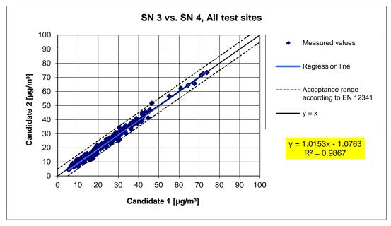
Figure 53: Result of parallel measurements with candidates SN 3 / SN 4, all test sites
