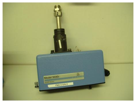
Figure 10: Model 5030i SHARP measuring system – Optics module
