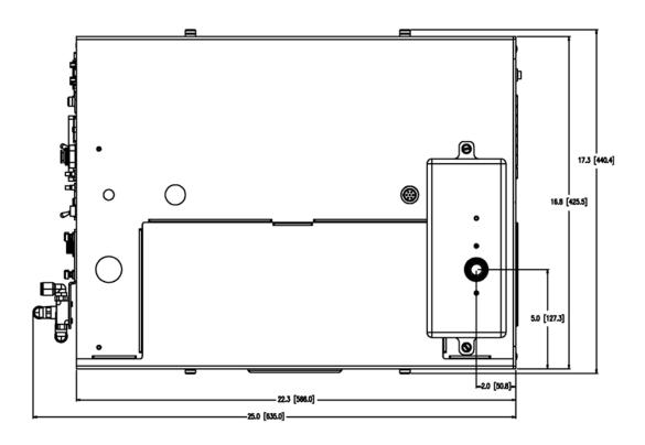
**Figure 2–4.** Model 5030*i* Top View—inches [millimeters]
