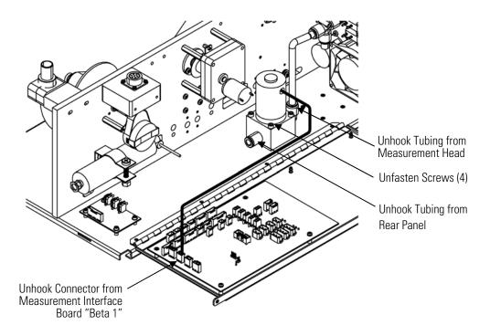
Figure 7–17. Replacing the Proportional Valve
