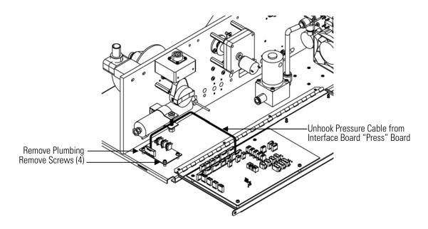
Figure 7–9. Replacing the Pressure Board Assembly
