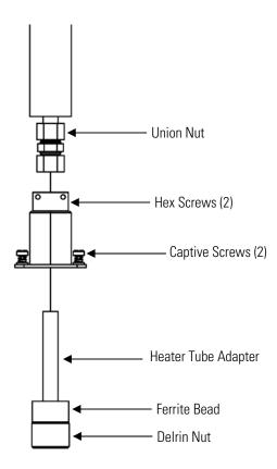
Figure 7–29. Replacing the Delrin Nut
