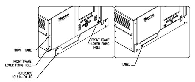
Figure 10-13. Front Panel Label Replacement
