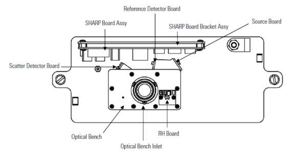
Figure 2: Hardware components Model 5030i SHARP – Optics module
