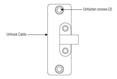
Figure 7–16. Replacing the Photo Interrupt Board
