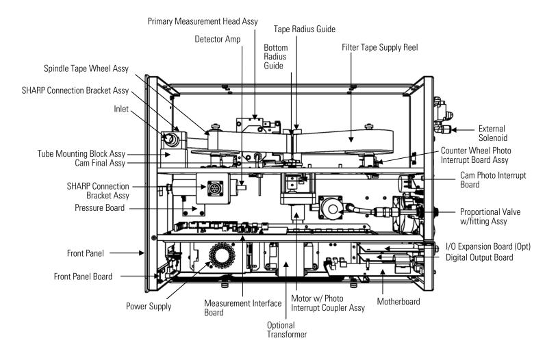
**Figure 7–2.** Model 5030*i* Component Layout
