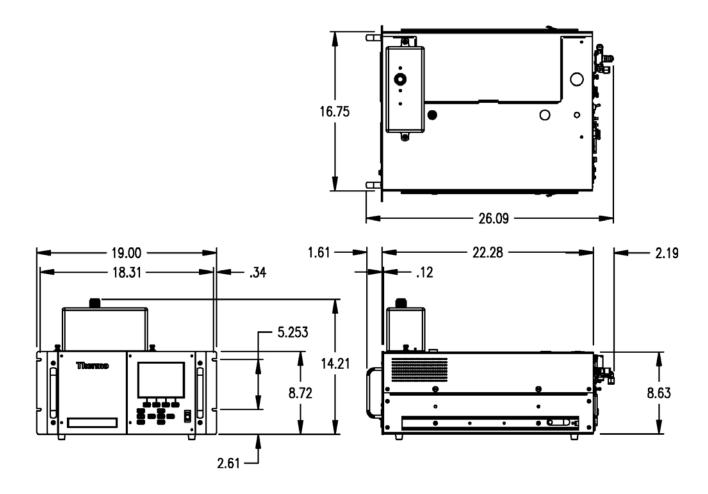
Figure 9–3. Retrofit Rack Mounting
