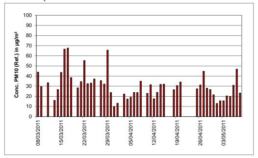
**Figure 19:** Course of PM<sub>10</sub> concentrations (reference) at the test site "Cologne, parking lot, winter"
