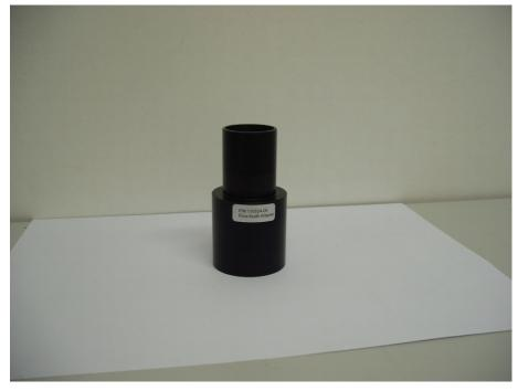
Figure 18: Leak test adapter
