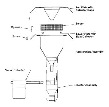
**Figure 5–1.** U.S. EPA PM<sub>10</sub> Inlet
