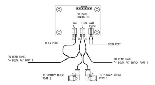
Figure 7–10. Replacing the Pressure Board Assembly Plumbing Connection
