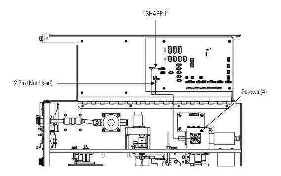
Figure 7–30. Replacing the Internal SHARP Cable Assembly
