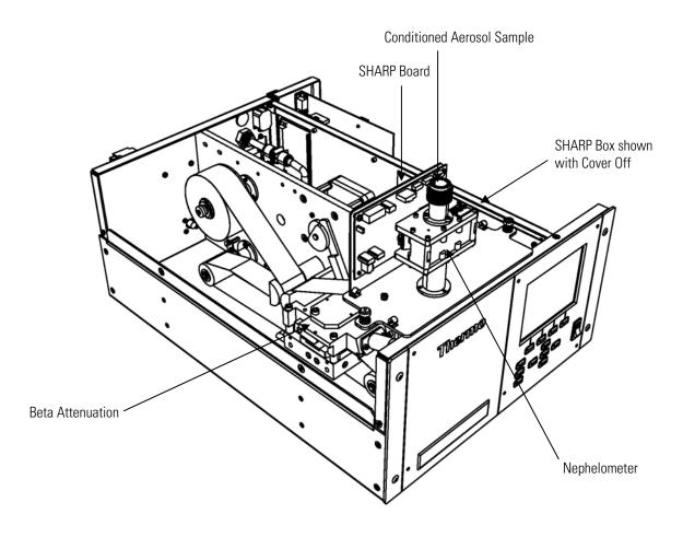
Figure 1–1. SHARP Monitor Sample Path
