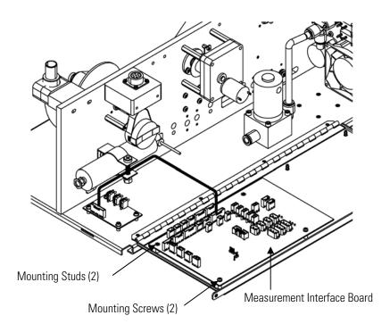
Figure 7–15. Replacing the Measurement Interface Board
