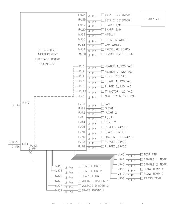
Figure 6-2. Board-Level Connection Diagram - Measurement System
