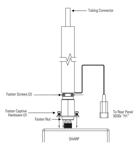
Figure 2–6. Heater Assembly
