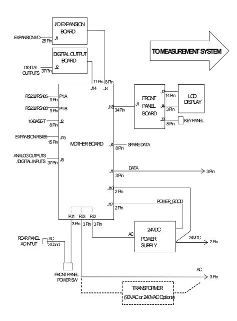
Figure 6-1. Board-Level Connection Diagram - Common Electronics
