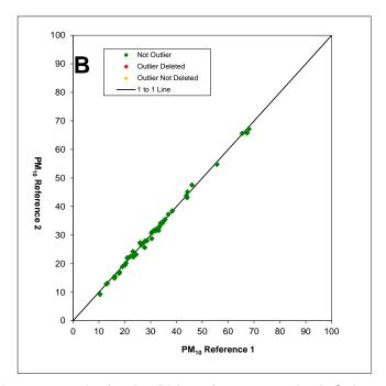
**Figure 28:** Grubbs test results for the PM<sub>10</sub> reference method, Cologne (winter)
