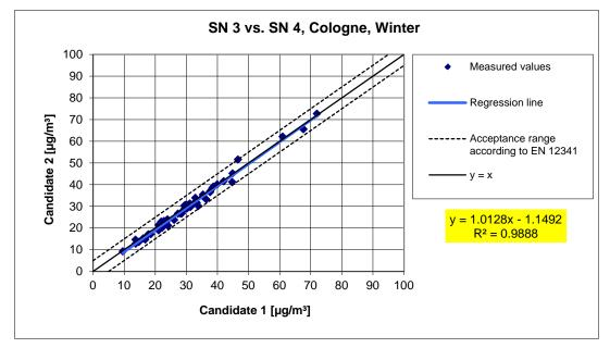
Figure 49: Result of parallel measurements with candidates SN 3 / SN 4, Cologne (winter)
