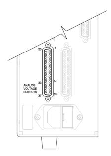
Figure 3-4. Pin-Out of Rear Panel Connector
