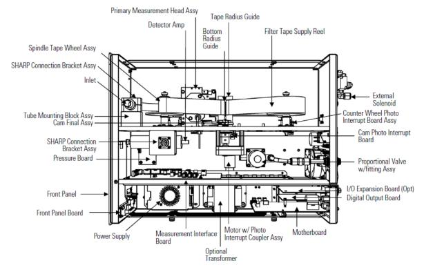
Figure 3: Hardware components Model 5030i SHARP – Beta module
