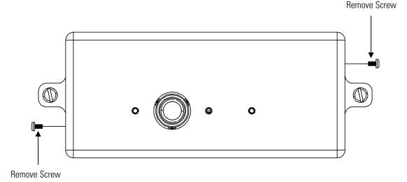
**Figure 7–24.** Removing the SHARP Optics Cover
