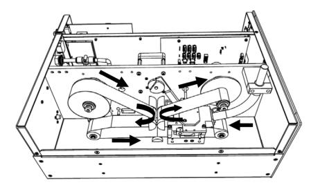
Figure 10–3. Filter Tape Installation Pathway
