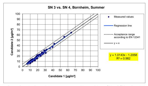
**Figure 50:** Result of parallel measurements with candidates SN 3 / SN 4, Bornheim (summer)
