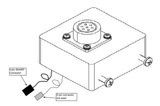
Figure 10–1. SHARP Optics Connection Bracket
