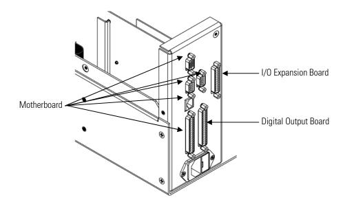
Figure 7–14. Rear Panel Board Connectors
