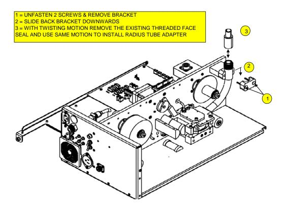
Figure 10–5. Radius Tube Adapter Install
