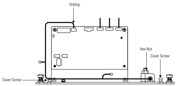
Figure 7–31. Replacing the Case Cable
