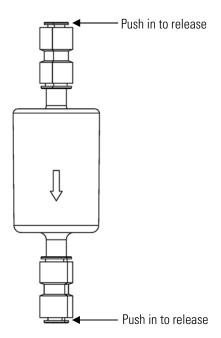
Figure 7–32. Replacing the External Zeroing Filter
