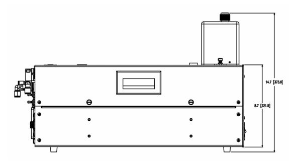
**Figure 2–3.** Model 5030*i* Side View—inches [millimeters]
