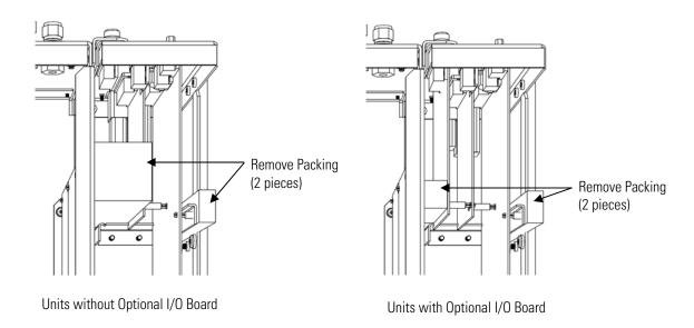
Figure 2–1. Remove the Packing Material
