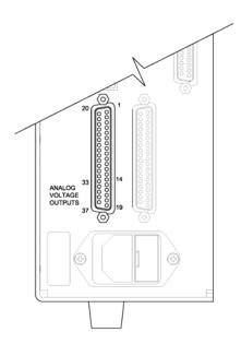
Figure 2-9. Pin-Out of Rear Panel Connector
