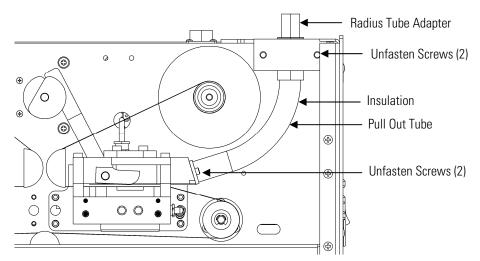
Figure 7–21. Replacing the Radius Tube
