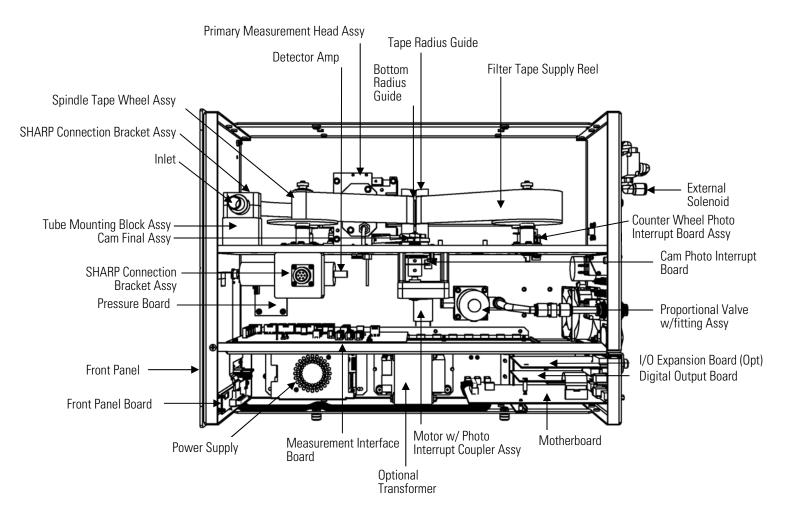
**Figure 8–1.** Model 5030*i* Hardware Components
