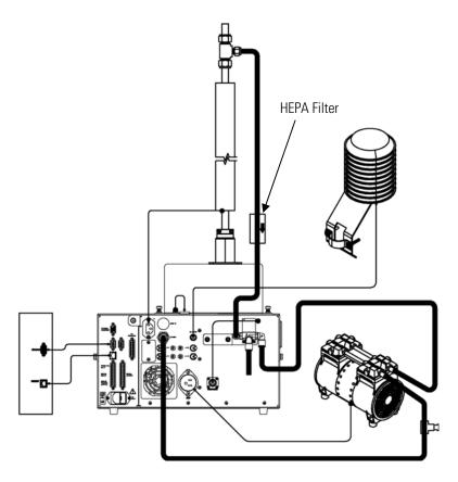
Figure 5–6. Replacing the External Pump Exhaust Filter
