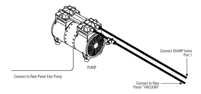
**Figure 7–8.** Replacing the Pump
