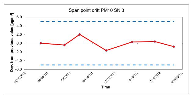
Figure 37: Drift of the measured value SN 3, measured component PM<sub>10</sub>
