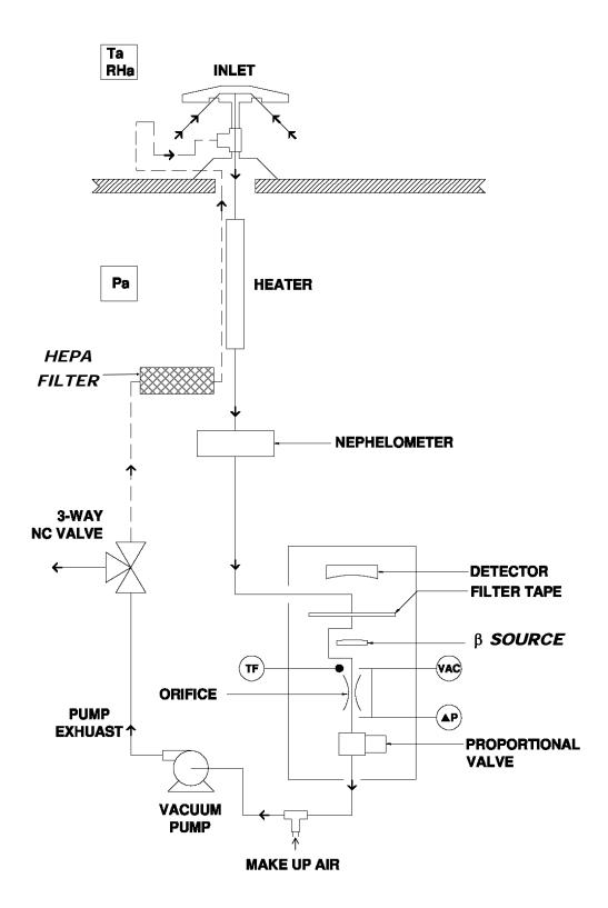
Figure 1–2. Nephelometer Sample and Zero Flow Schematic
