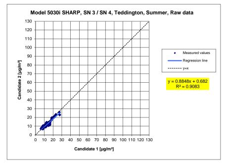
**Figure 60:** Results of the parallel measurements with the candidates SN 3 / SN 4, measured component PM<sub>10</sub>, test site Teddington (summer)
