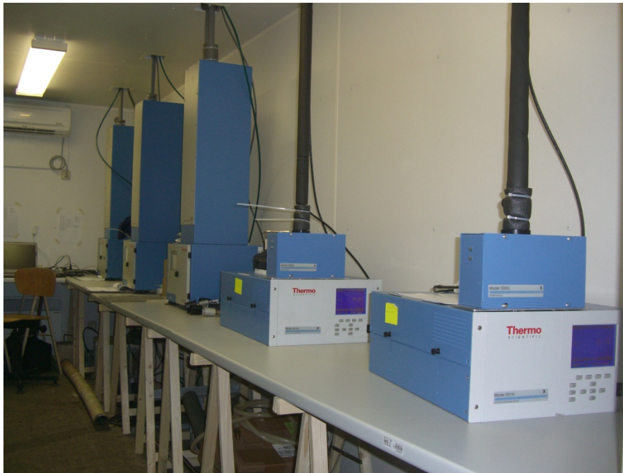
Figure 12: Model 5030i SHARP measuring system (Systems 1 and 2 from right) at measuring station
