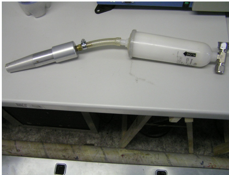
Figure 16: Zero filter for supplying air free of suspended particles and its connection adapter
