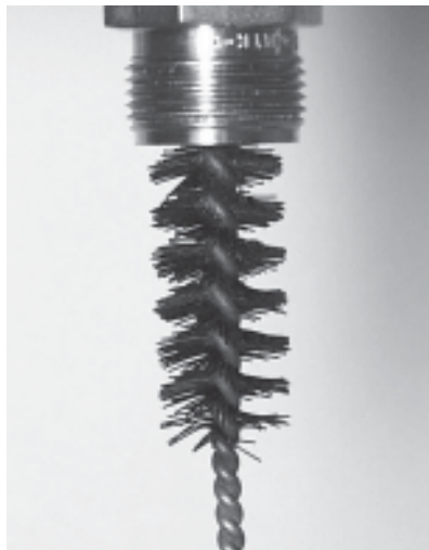
Figure 5-47. Cleaning the valve with the valve brush.
