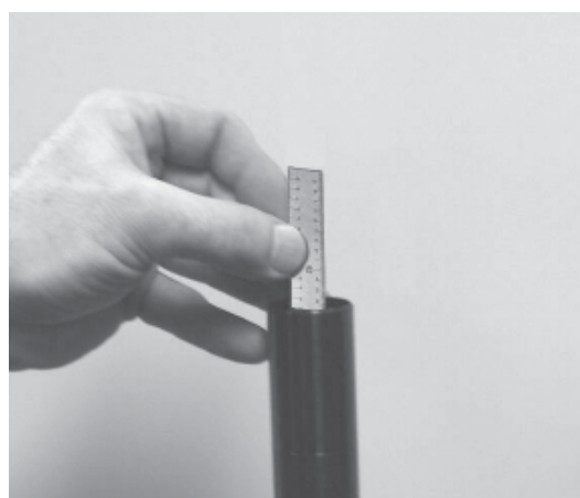
Figure 2-7. Measuring the distance from the top of the sample tube to the top of the flow splitter.
