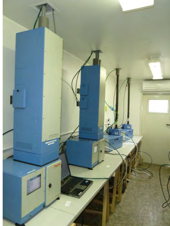
Figure 7: Measuring device TEOM 1405-DF Ambient Particulate Monitor (2 nd system from left) in measuring station
