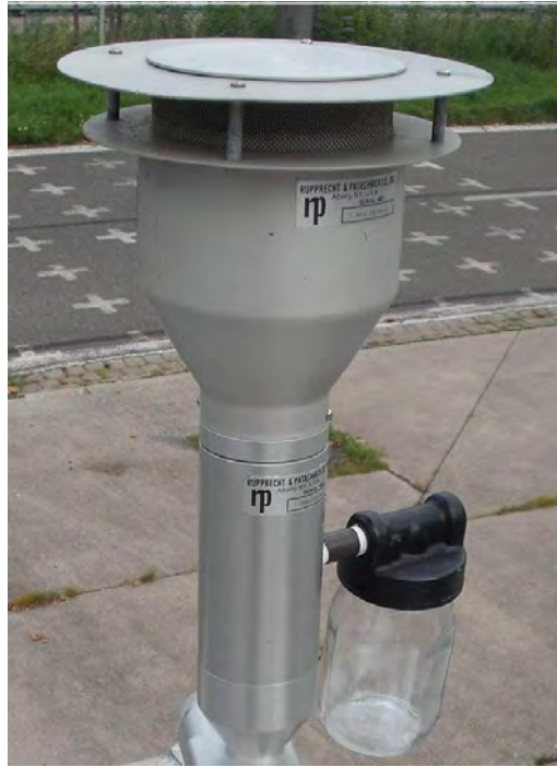
Figure 3: American PM 10 -sampling inlet (Original style, p/n 57-000596-0001) for TEOM 1405-DF Ambient Particulate Monitor
