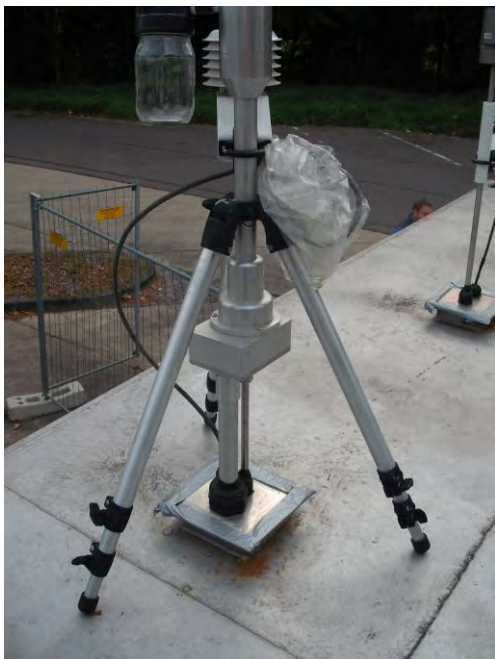
Figure 4: Virtual impactor (p/n 55-010164) for TEOM 1405-DF Ambient Particulate Monitor
