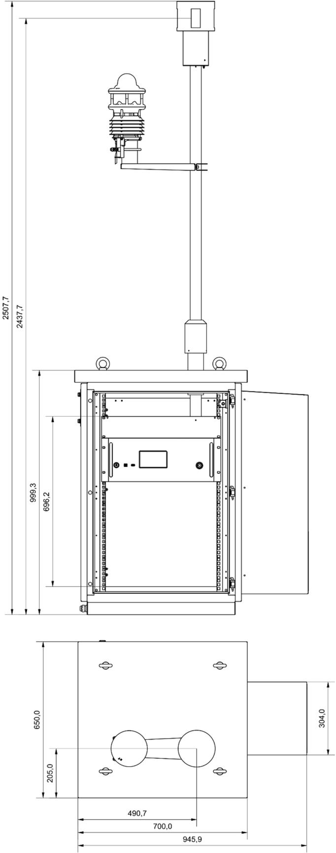
Position of the sample inlet in the 19" module, with scale
