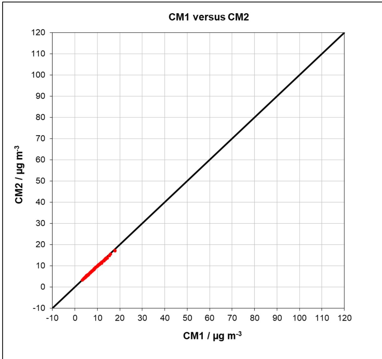
Figure 36: Results of parallel measurements, Cologne, PM<sub>2.5</sub>
