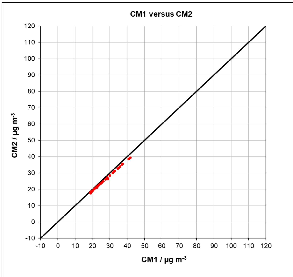
Figure 44: Results of parallel measurements, all sites  $\geq 18 \mu\text{g/m}^3$ , PM<sub>2.5</sub>
