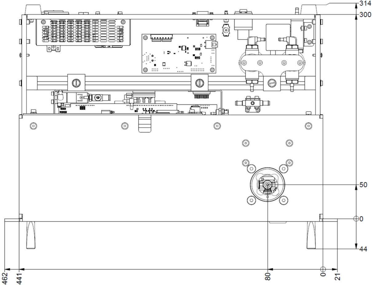
EDM 280 roof flange with alignment aid
