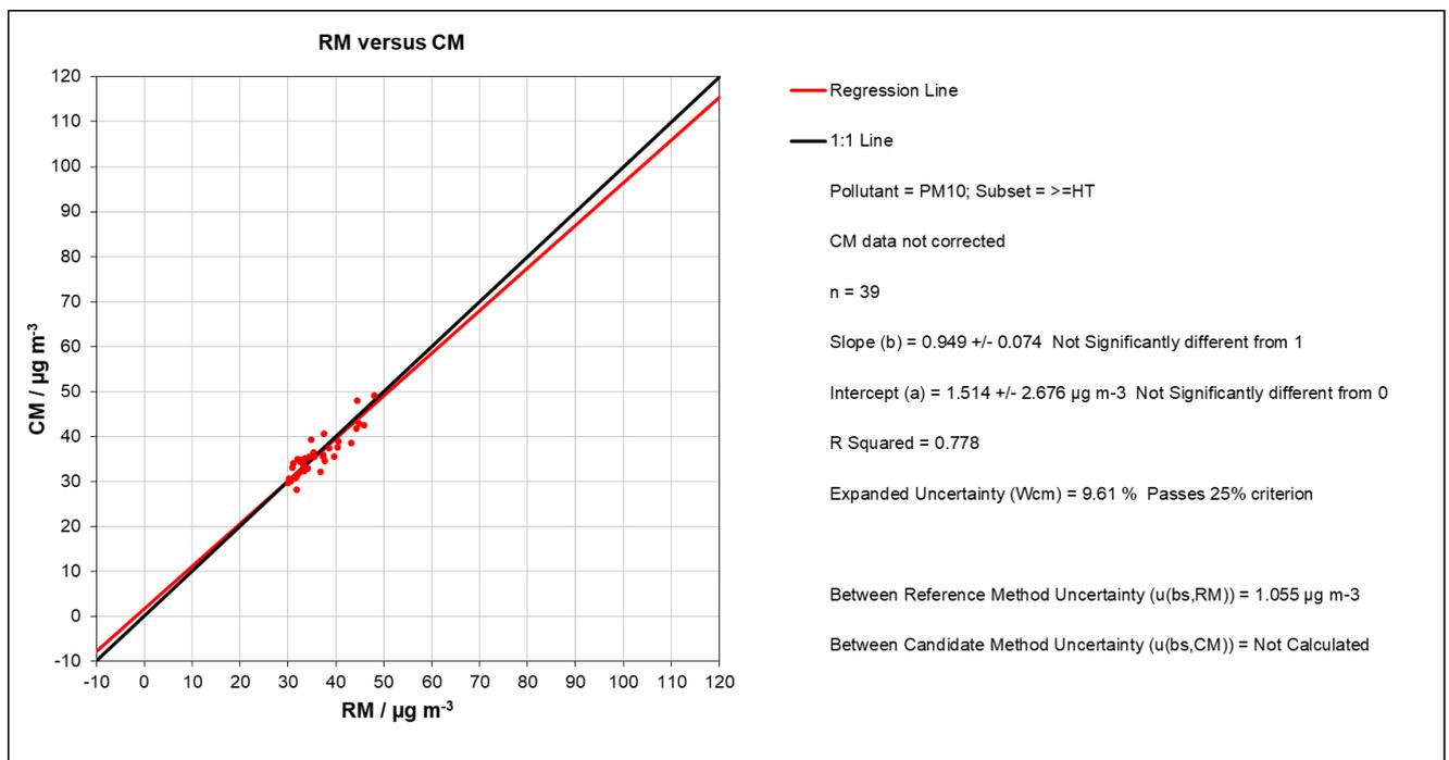
Figure 71: Reference vs candidate, SN FE114, all sites ≥30 µg/m<sup>3</sup>, PM<sub>10</sub>
