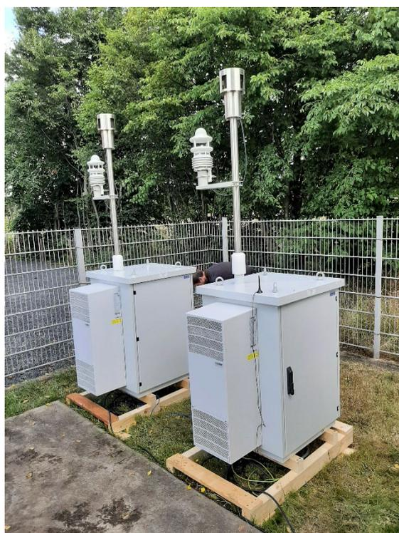
Figure 9: Fully air-conditioned, weatherproof housing Model 199
