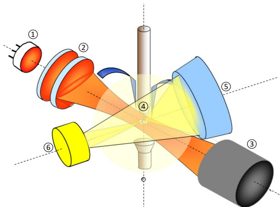
Figure 3-2: Schematic structure of the optical measuring cell
