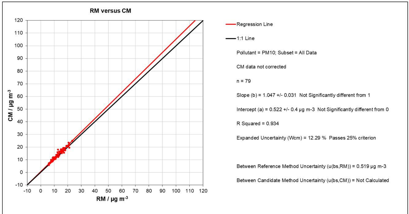
Figure 62: Reference vs candidate, SN FE111, Cologne, PM<sub>10</sub>
