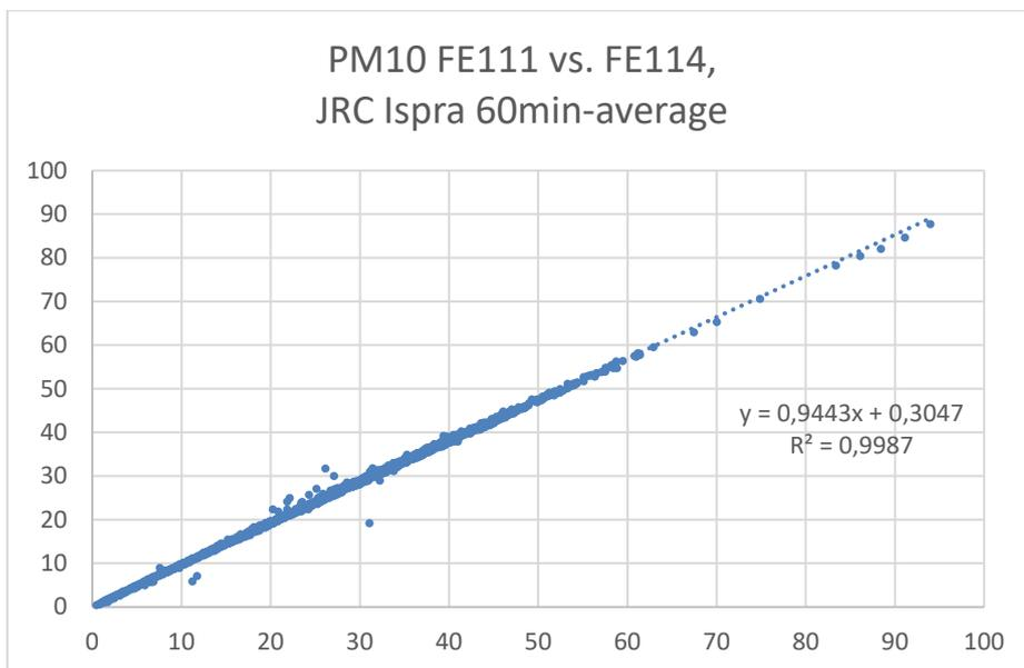
Figure 30: Comparison FE111 vs FE114, PM<sub>10</sub>, JRC Ispra, 60 min measuring interval
