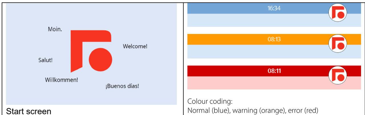
Figure 5-3: Touch display start screen and colour coding
