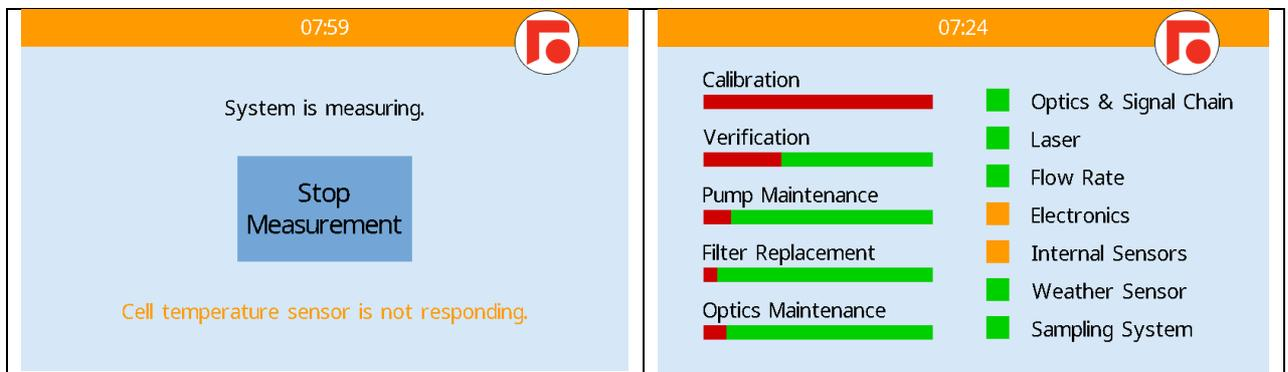
Figure 5-13: Touch display example, warning colour code
