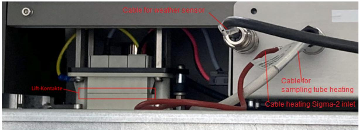
Figure 5-2: Back of sampling tube holder with lift contact and connected cables
