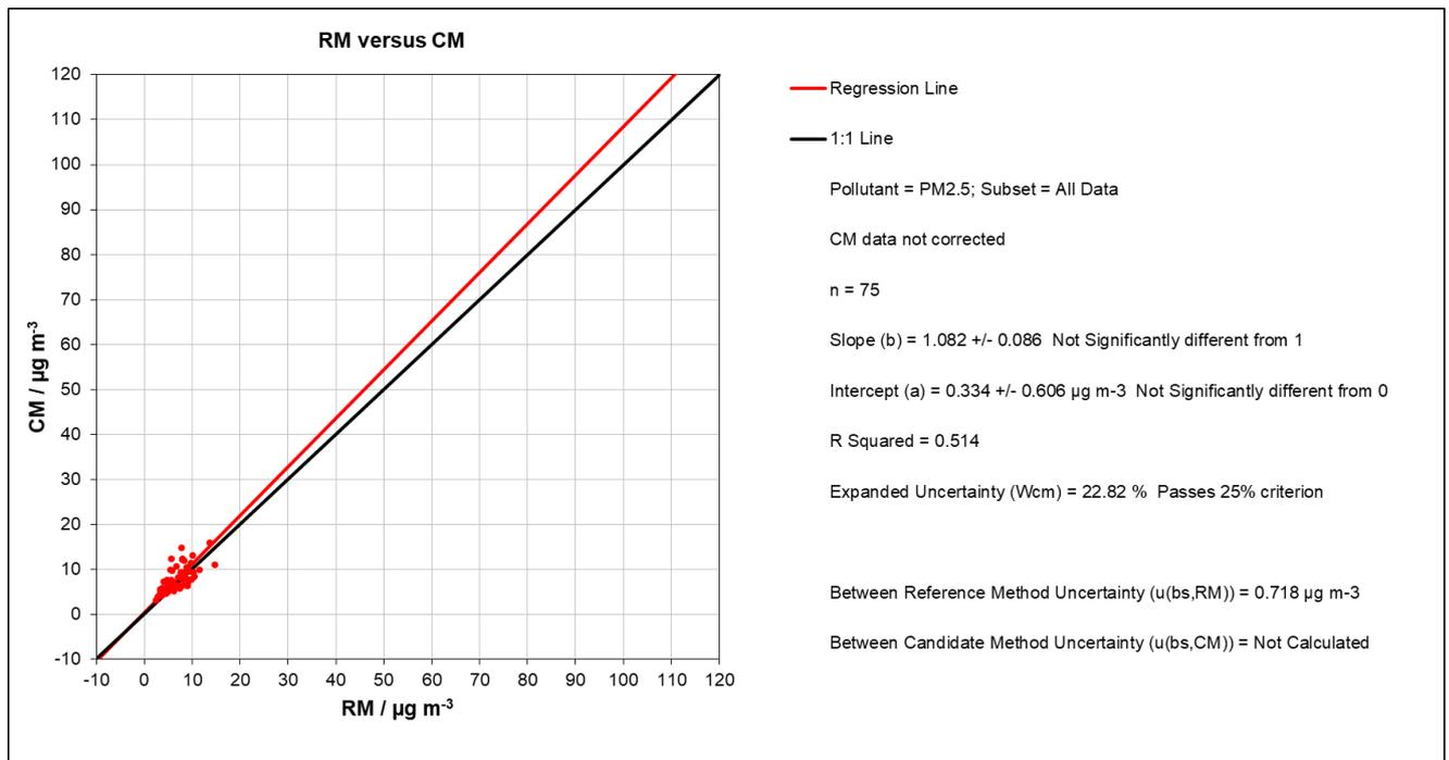
Figure 55: Reference vs candidate, SN FE114, Niederzier, PM<sub>2.5</sub>
