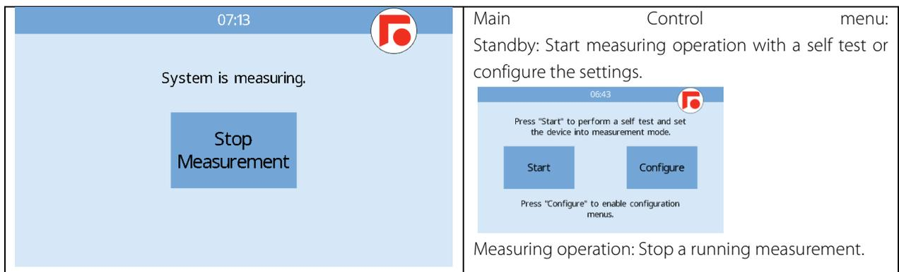
Figure 5-6: Stop measurements or configure settings
