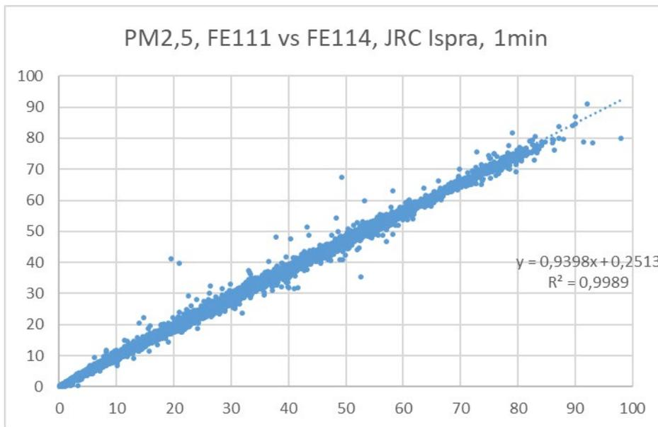
Figure 32: Comparison FE111 vs FE114, PM<sub>2.5</sub>, JRC Ispra, 1 min measuring interval
