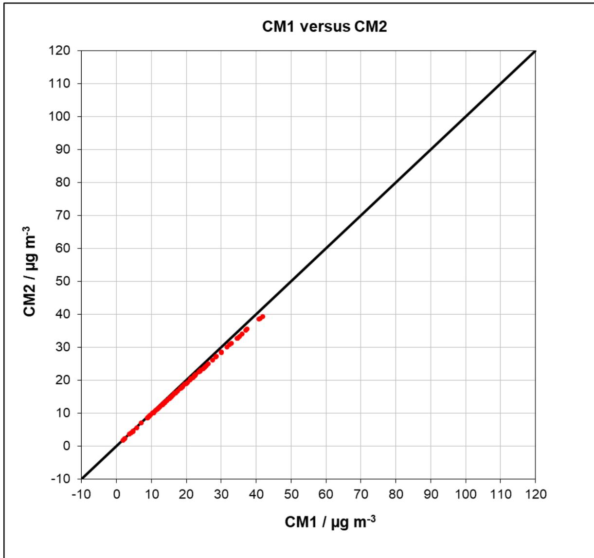
Figure 42: Results of parallel measurements, JRC Ispra, PM<sub>2.5</sub>
