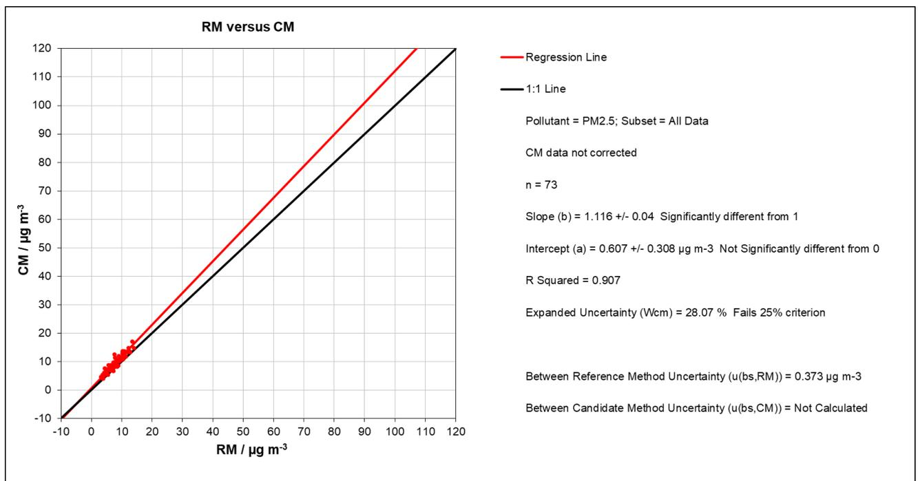
Figure 51: Reference vs candidate, SN FE114, Cologne, PM<sub>2.5</sub>
