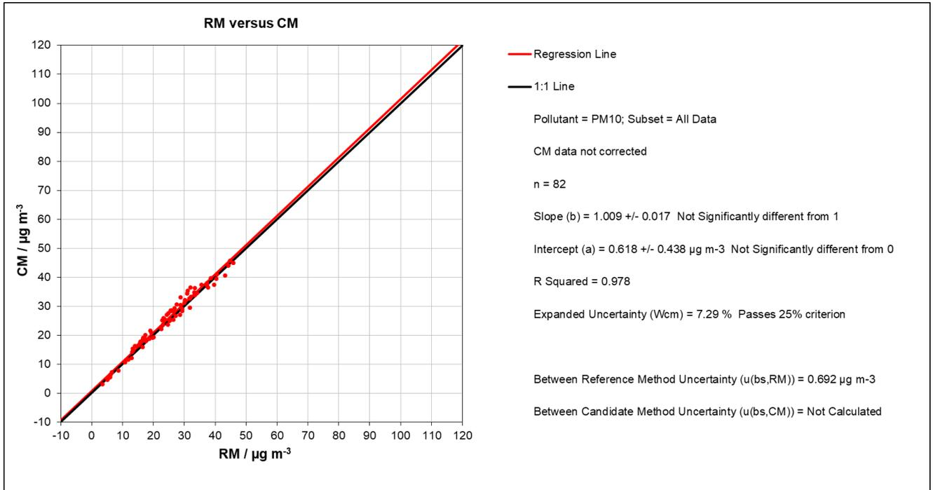
Figure 68: Reference vs candidate, SN FE111, JRC Ispra, PM<sub>10</sub>
