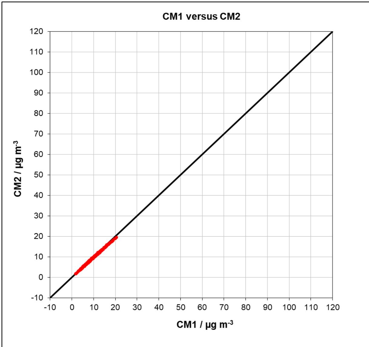
Figure 46: Results of parallel measurements, all sites < 18 µg/m<sup>3</sup>, PM<sub>2.5</sub>
