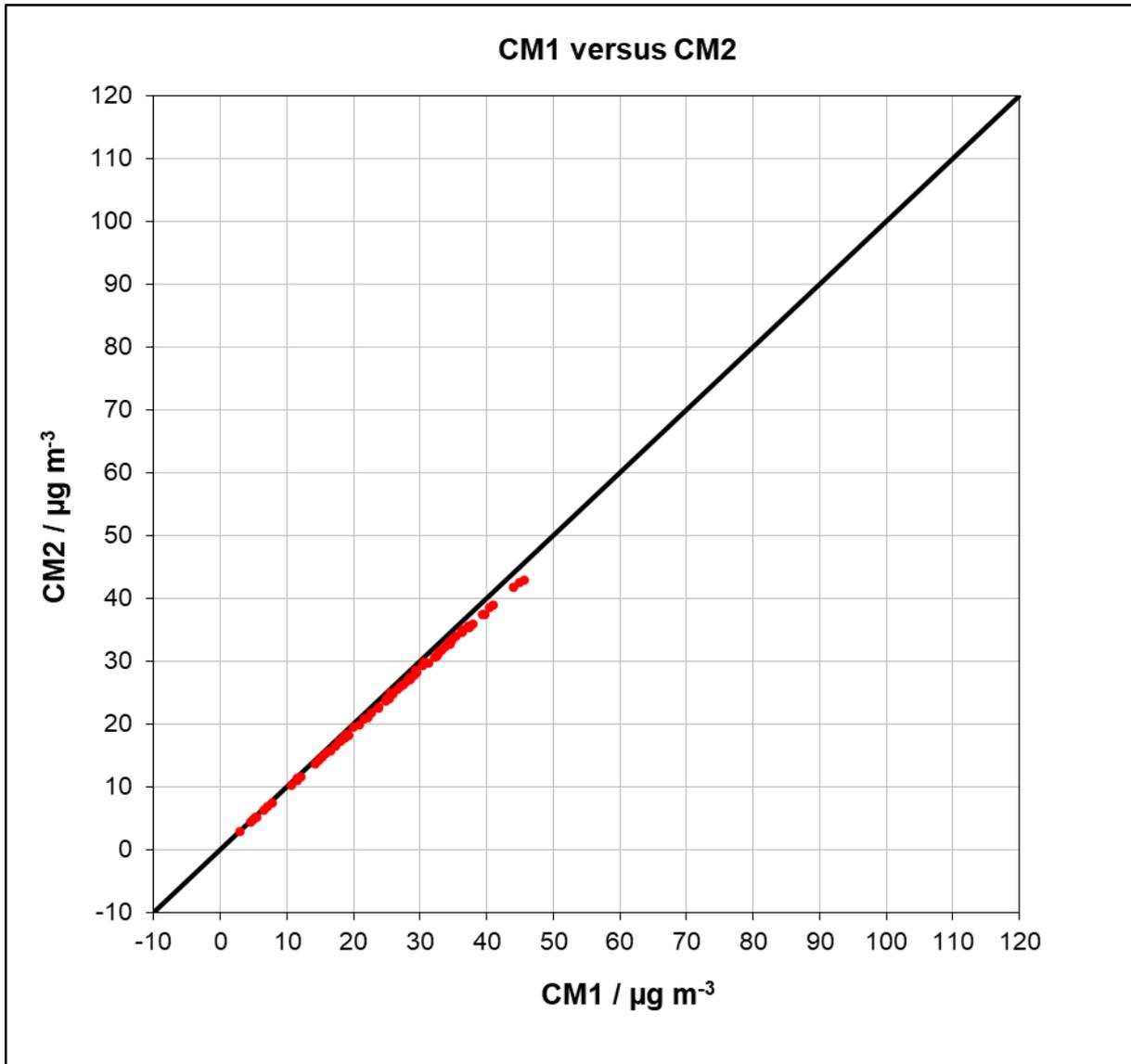
Figure 43: Results of parallel measurements, JRC Ispra, PM<sub>10</sub>
