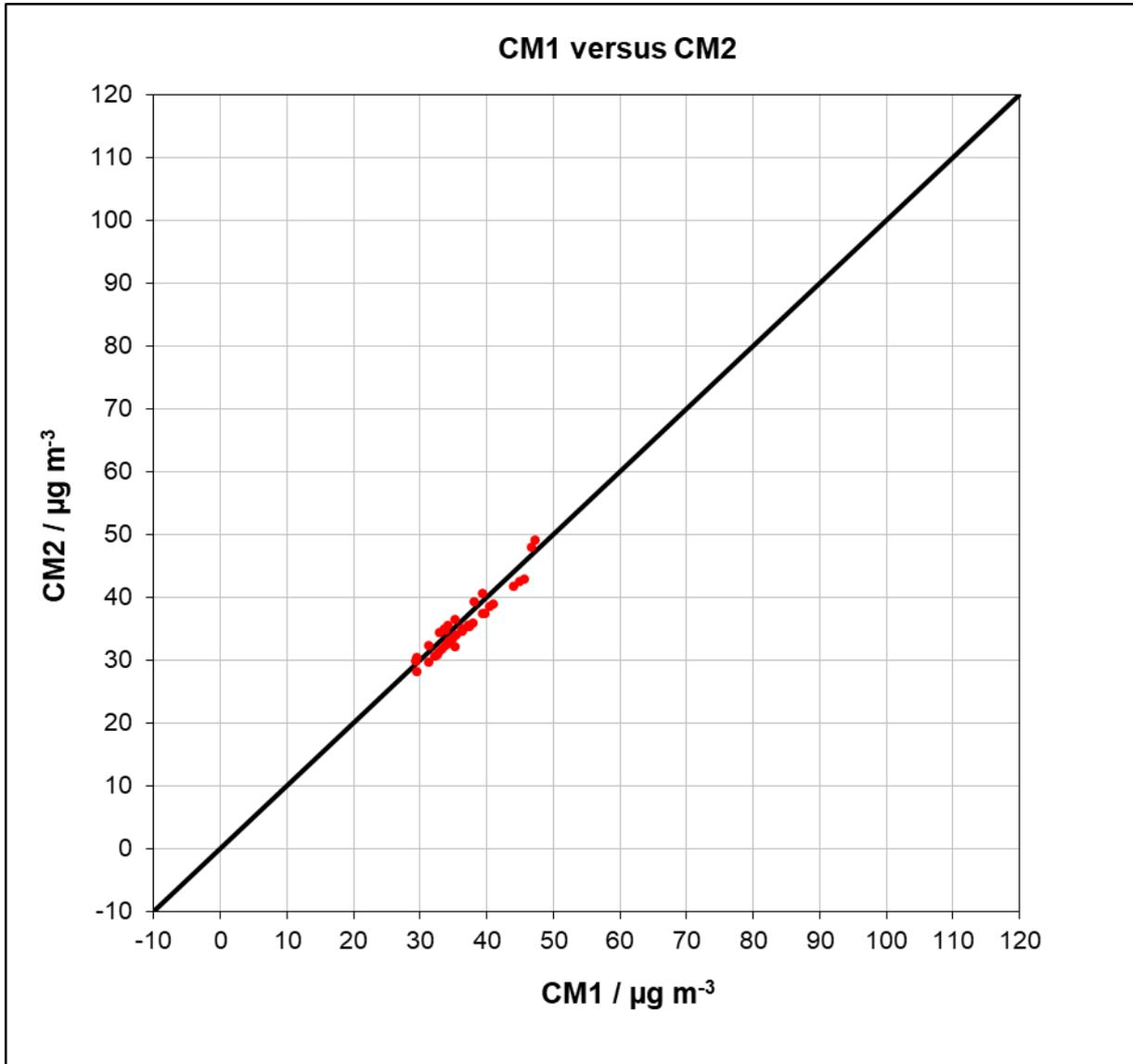
Figure 45: Results of parallel measurements, all sites ≥ 30 µg/m<sup>3</sup>, PM<sub>10</sub>
