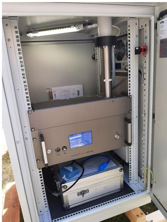
Figure 4: Sampling tube holder + measuring module in housing Modell 199
