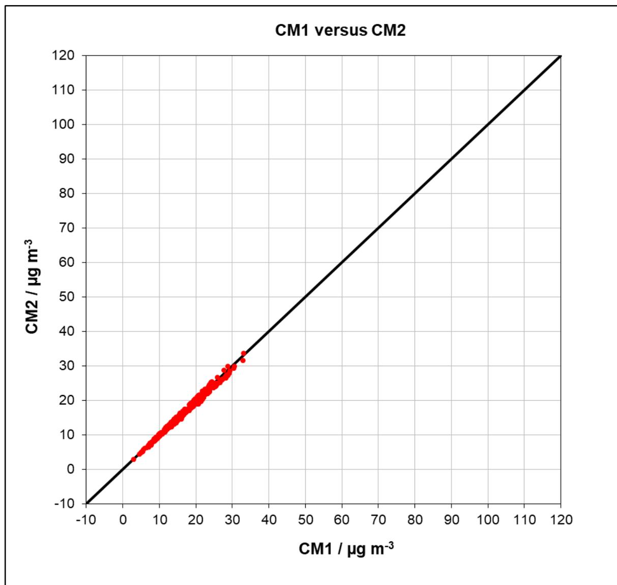
Figure 47: Results of parallel measurements, all sites < 30 µg/m<sup>3</sup>, PM<sub>10</sub>
