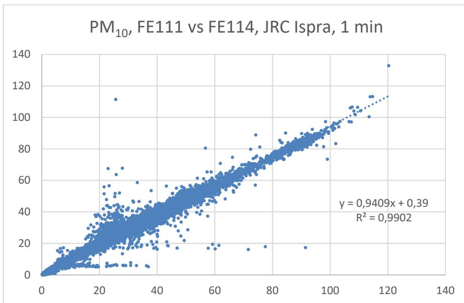
Figure 29: Comparison FE111 vs FE114, PM<sub>10</sub>, JRC Ispra, 1 min measuring interval
