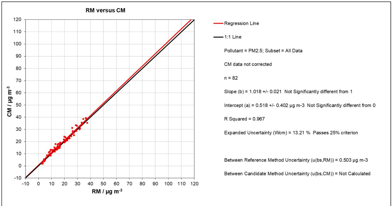
Figure 57: Reference vs candidate, SN FE114, JRC Ispra, PM<sub>2.5</sub>
