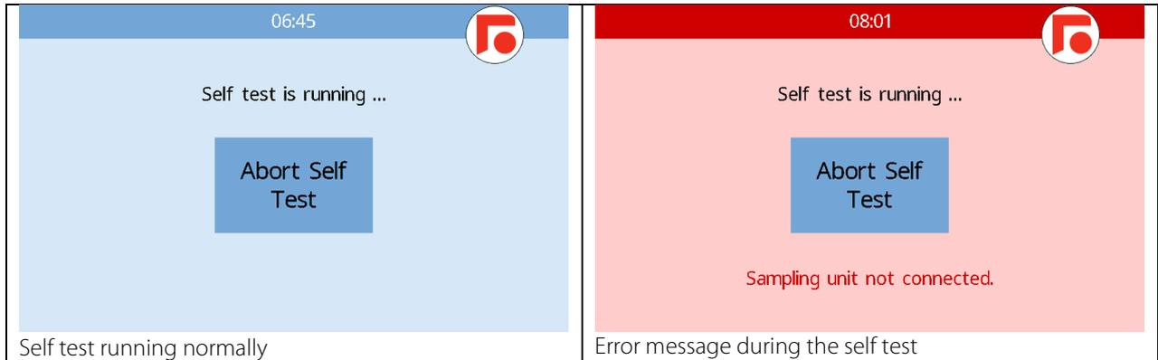
Figure 5-5: Normal self test and self test with error message
