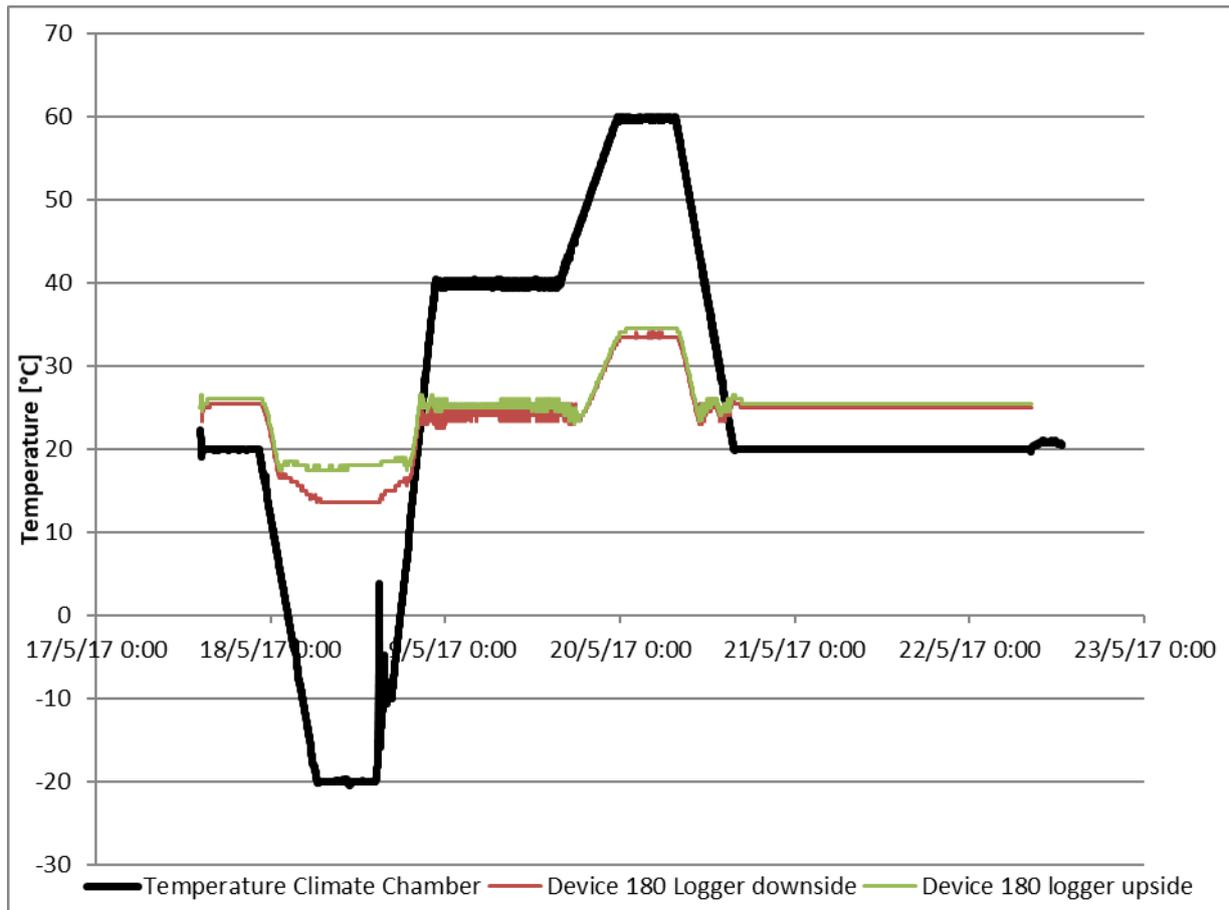
Figure 10: Temperature profile, climate chamber test Model 199
