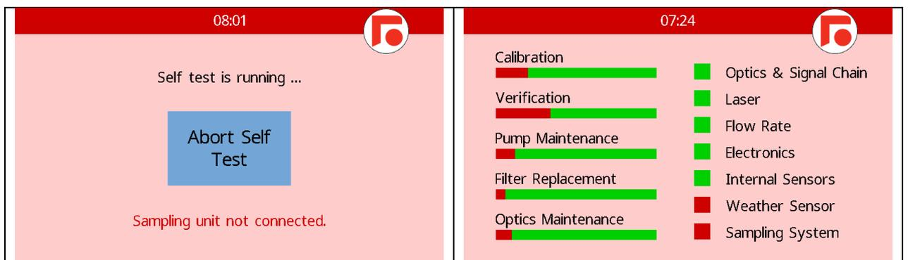
Figure 5-14: Touch display example, error colour code
