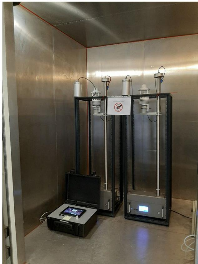
Figure 11: EDM 280 in climatic chamber, dispenser connected to sample inlet
