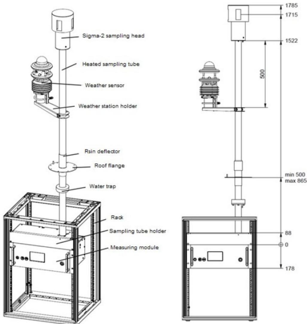
Figure 2: Schematic structure of the EDM 280
