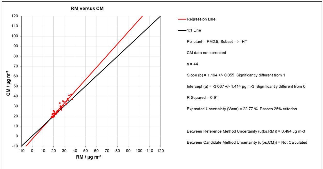
Figure 58: Reference vs candidate, SN FE111, all sites  $\geq 18 \mu\text{g}/\text{m}^3$ , PM<sub>2.5</sub>
