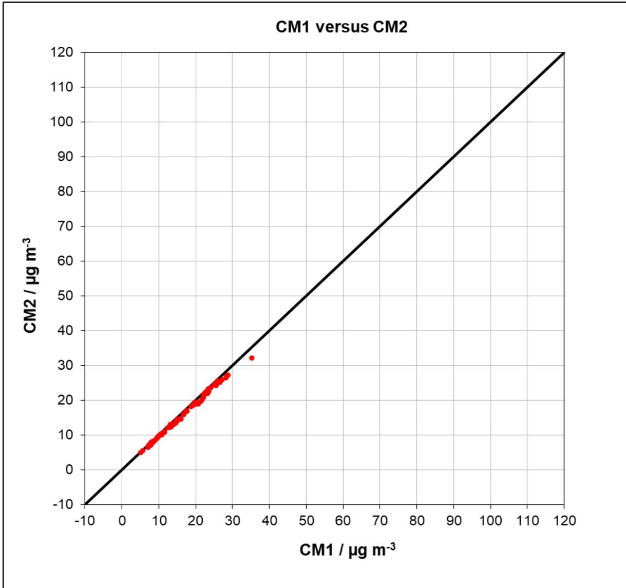
Figure 39: Results of parallel measurements, Bornheim, PM<sub>10</sub>
