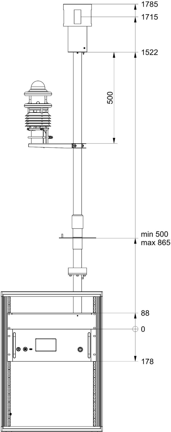
Complete system in fully air-conditioned, weatherproof housing for model 199 19" device (item number 4025195), with scale
