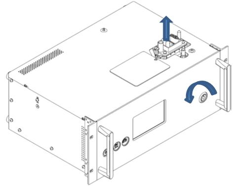
Figure 4-5: Measuring module with lift extended (closed position)
