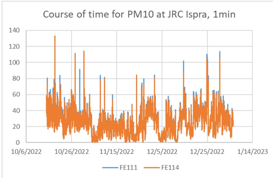
Figure 28: PM<sub>10</sub> concentrations, JRC Ispra, 1 min measuring interval
