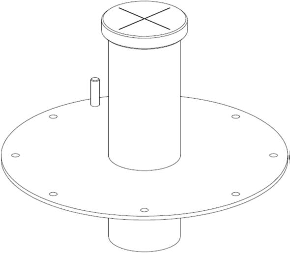
Measuring module and sampling tube holder with optional data logger
