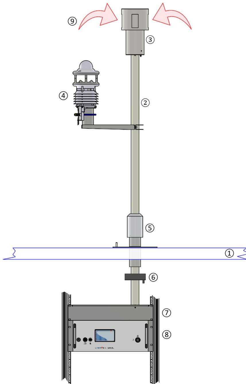
Figure 3-1: Schematic structure of the EDM 280
