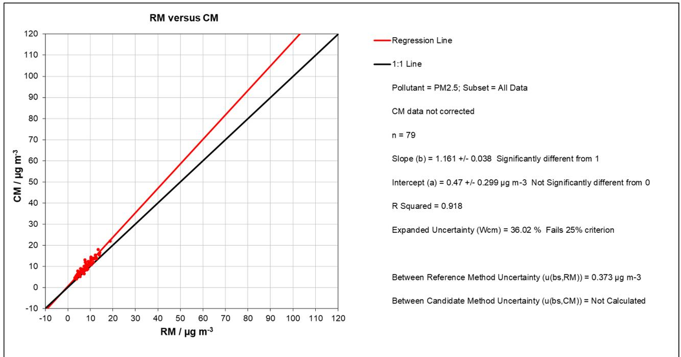
Figure 50: Reference vs candidate, SN FE111, Cologne, PM<sub>2.5</sub>
