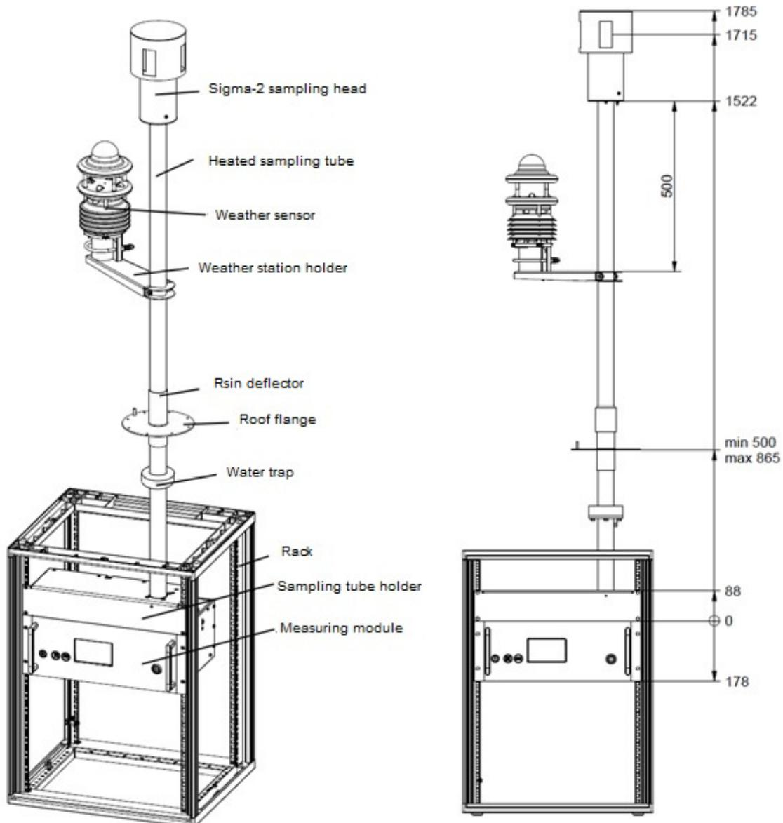
Figure 5-1: Overall view of the EDM 280 system
