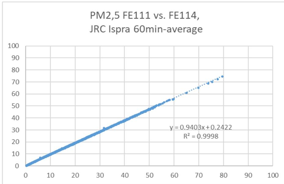
Figure 33: Comparison FE111 vs FE114, PM<sub>2.5</sub>, JRC Ispra, 60 min measuring interval
