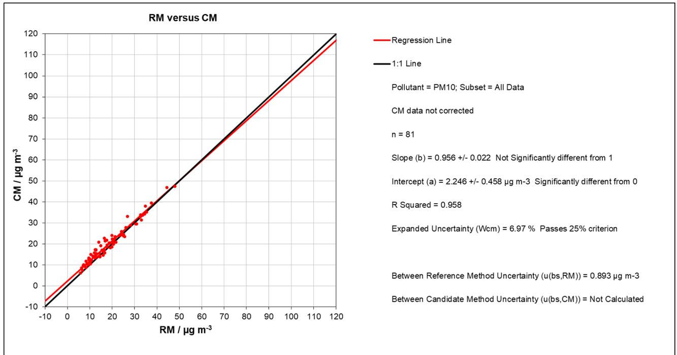
Figure 66: Reference vs candidate, SN FE111, Niederzier, PM<sub>10</sub>
