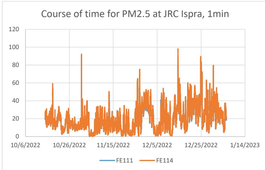
Figure 31: PM<sub>2.5</sub> concentrations, JRC Ispra, 1 min measuring interval
