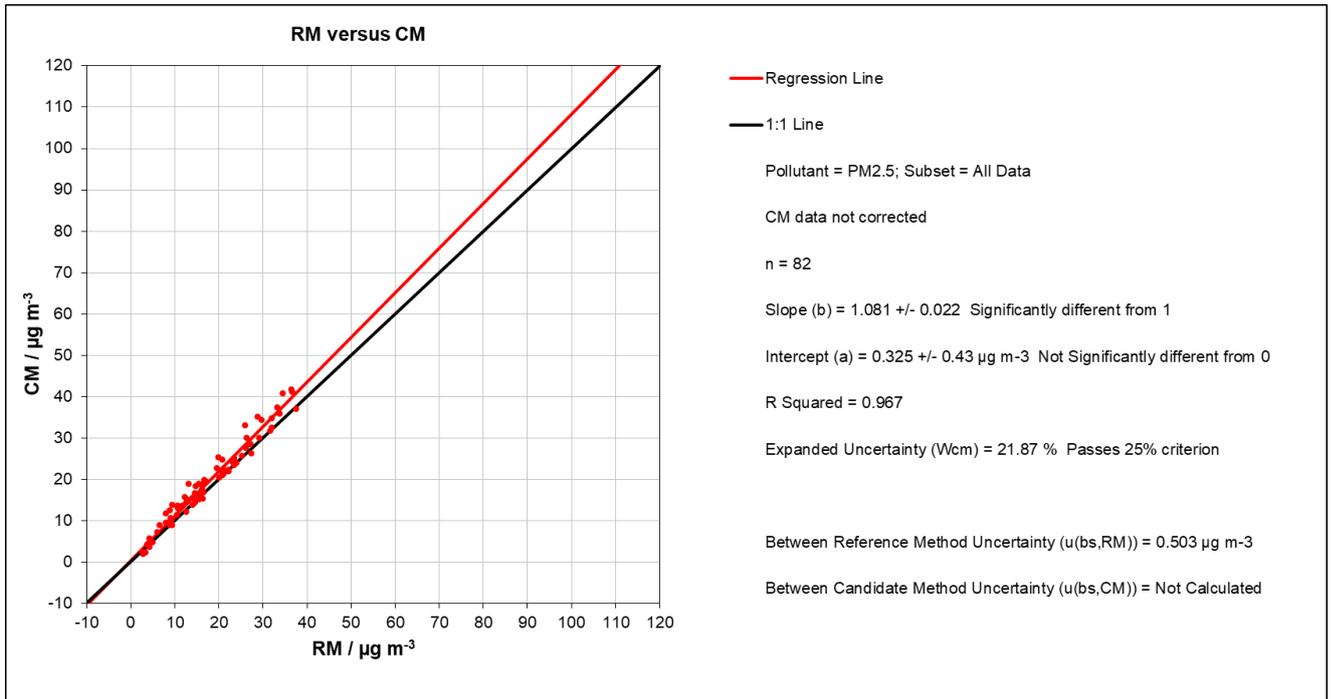
Figure 56: Reference vs candidate, SN FE111, JRC Ispra, PM<sub>2.5</sub>
