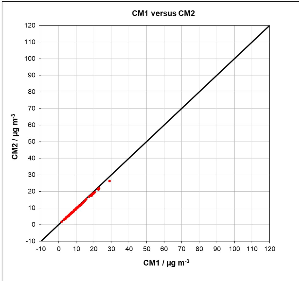
Figure 38: Results of parallel measurements, Bornheim, PM<sub>2.5</sub>
