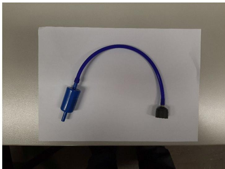
Figure 7: Adapter for sample inlet with mounted zero air filter
