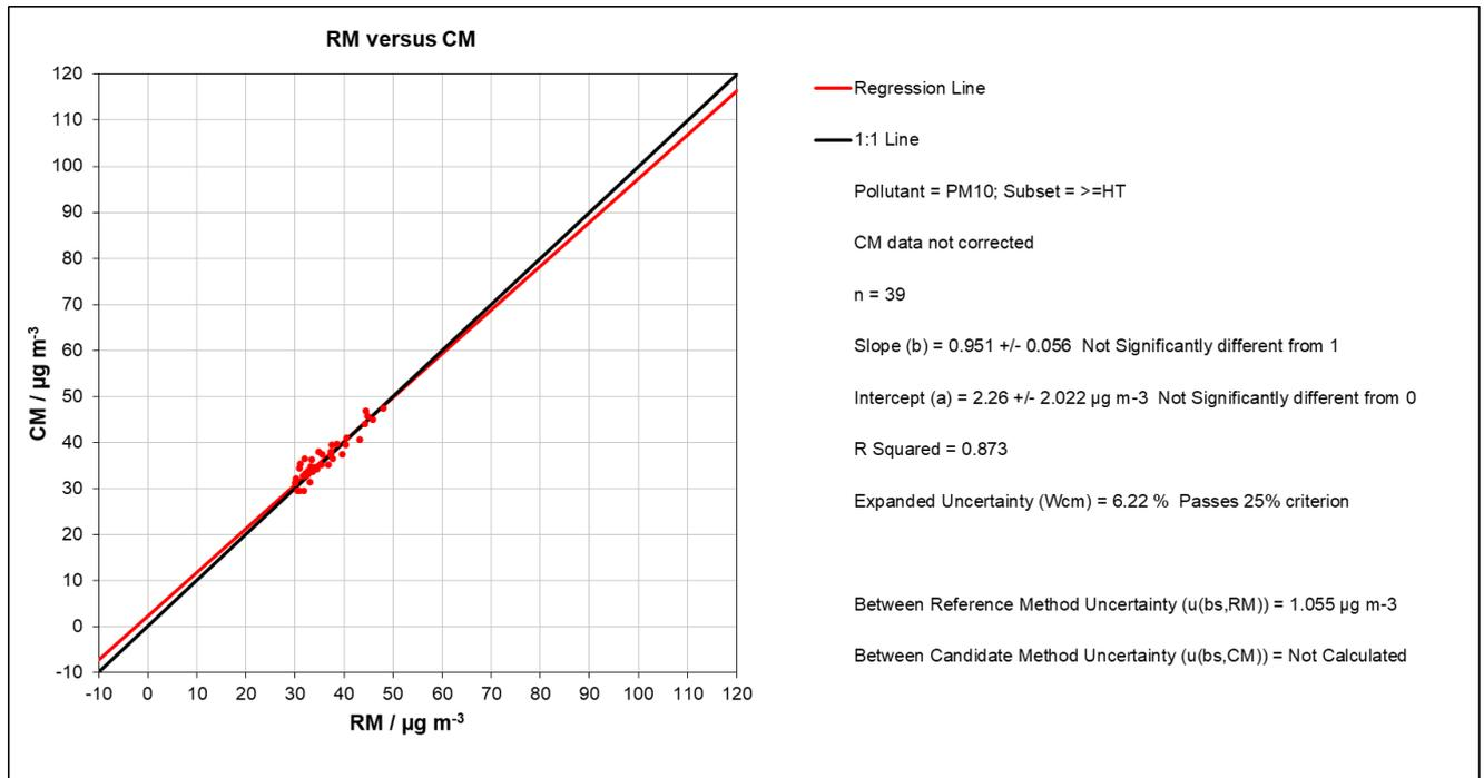
Figure 70: Reference vs candidate, SN FE111, all sites ≥30 µg/m<sup>3</sup>, PM<sub>10</sub>
