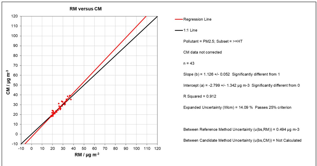
Figure 59: Reference vs candidate, SN FE114, all sites  $\geq 18 \mu\text{g}/\text{m}^3$ , PM<sub>2.5</sub>
